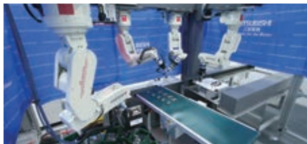
Robot system for placing parts discretely
