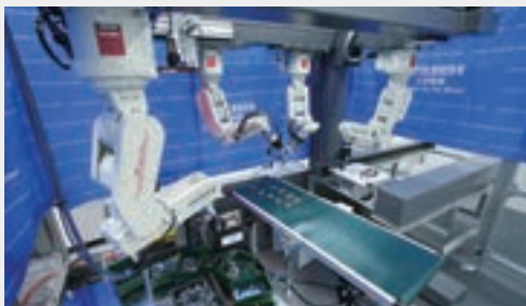
Robot system for placing parts discretely
